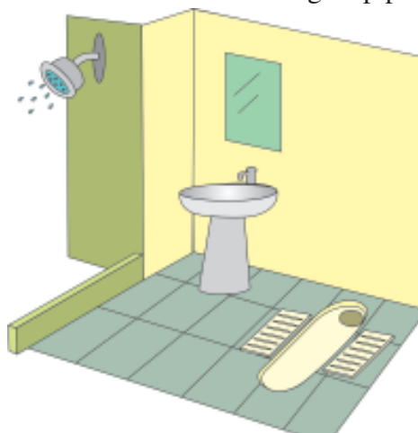
Fig.12.20: A squatting pan water closet
